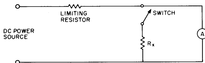
Figure 13—Ammeter Method of Resistance Measurement
